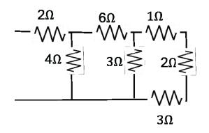
**Example 3**: **a**) Find the equivalent resistance of the circuit shown below. **b**) Find the currents through each resistor if a 14-V battery is connected to the circuit. **c**) Find the total power dissipated in the circuit.
